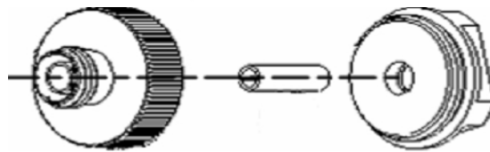
Structure of optical port
